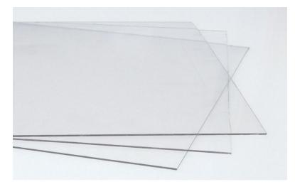
Plastic glazing will be used in the Behavioral Health areas of the Wynn Hospital. It is made up of a polycarbonate sheet with a proprietary abrasion/UV resistant coating that approaches glass in performance. This coating is graffiti resistant and paint, adhesives and other materials will not adhere to its surface. Also, its impact resistance is 30 times higher than acrylic sheets and 100 times stronger than tempered glass.
